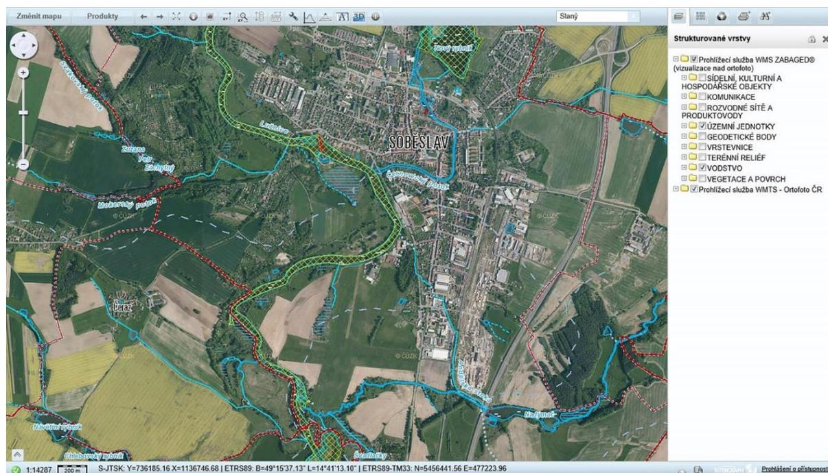
Orthophoto CR is provided in datasets on map sheets of the State map 1: 5 000, further via viewing services and in the printed form. Data are in raster format JPEG or TIFF since 2016 with the resolution of 0.20 m on the ground and are georeferenced in the coordinate system S-JTSK. The data sets for coordinate system WGS 84 are also provided.
