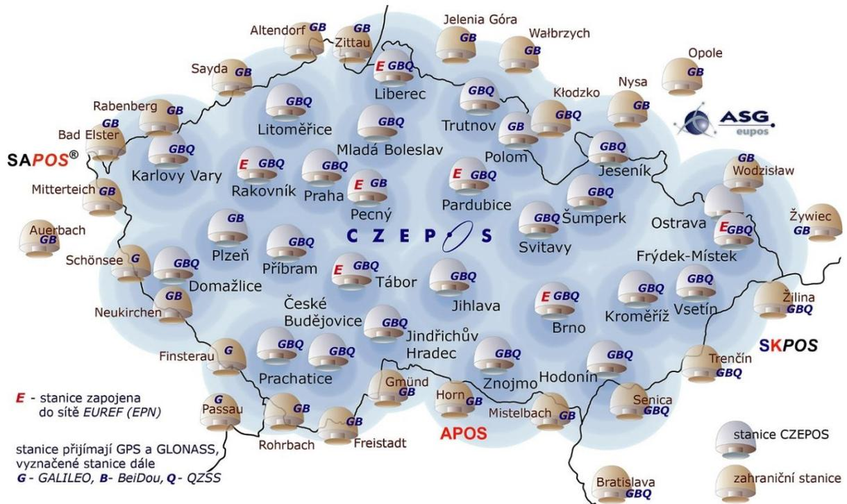
In 2019 the modernization of CZEPOS receivers was completed. CZEPOS services are at present compatible with all accessible satellite systems, i.e. American navigation satellite system NAVSTAR GPS, Russian global navigation satellite system GLONASS, European navigation satellite system Galileo, Chinese BeiDou system as well as with regional Japanese QZSS.
